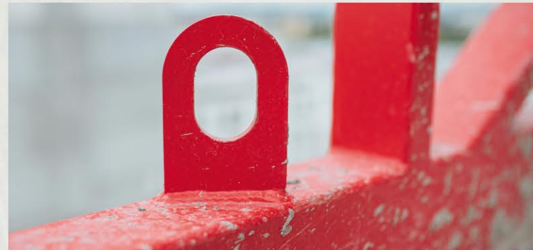
Fixing of the crane's sling.
