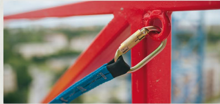
anchoring points for PPE
